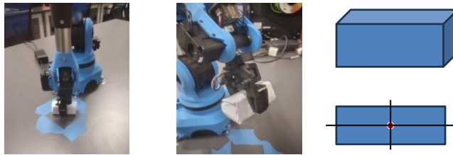
Fig. 1. The robotic gripper is capable of lifting trash object.
