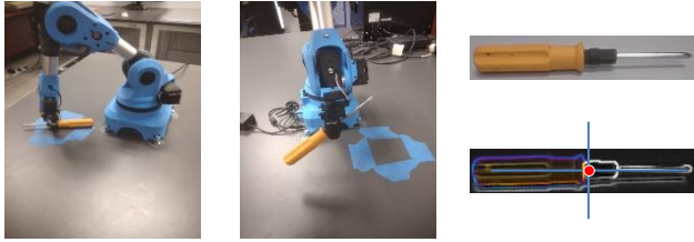
Fig. 3. Robotic grippers are not able to lift trash objects perfectly.
