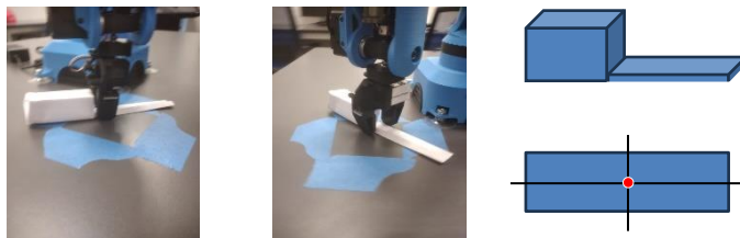
Fig. 2. The robotic gripper is unable to grip or lift trash object.
