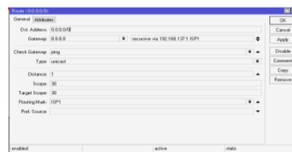
Figure 3. Configuring Check Gateway and Routing Mark on ISP1
