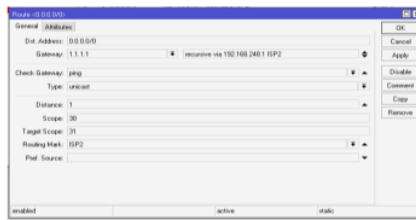
Figure 4. Configuring Check Gateway and Routing Mark on ISP2
