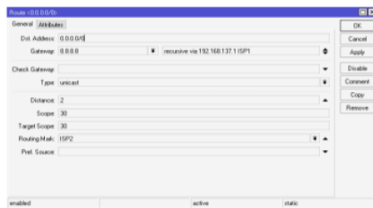
Figure 5. Configuring Routing Mark as Backup Gateway from ISP1
