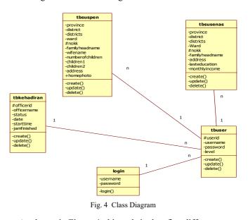
As shown in Figure 4, this website has five different types of tables that can store the website's database. tbsuspen, tbsusenas, tbkehadiran, tbuser, and login are the names of the tables. All of the tables in the website system are linked together so that the system can store and retrieve the database as efficiently as possible. Table tbsuspen is the one with the most users. Table 2 shows the cardinality of each table with the other table in detail:
