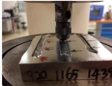
FIGURE 5. Hardness test on the stir zone of the FSP.
