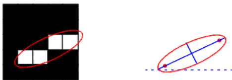
Fig. 7 Representation of the region with the ellipse approach
