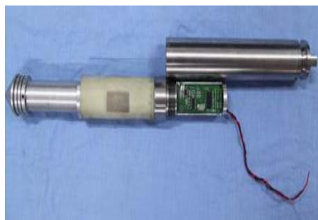
Figure 2. Hollow Inclusion Strain Cell Tool with Data Collector Automatic of Overcoring Techniques [3]
