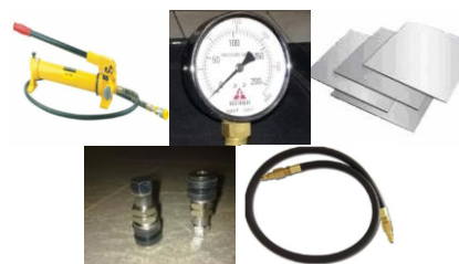
Figure 7. Flat Jack Making Tools and Materials [7]
