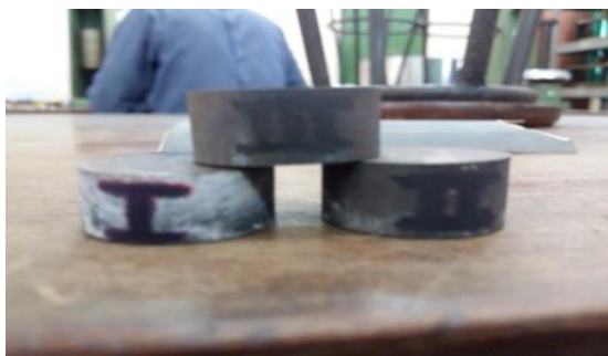
Figure 5. Specimen after Treatment of Carburizing Pack.
