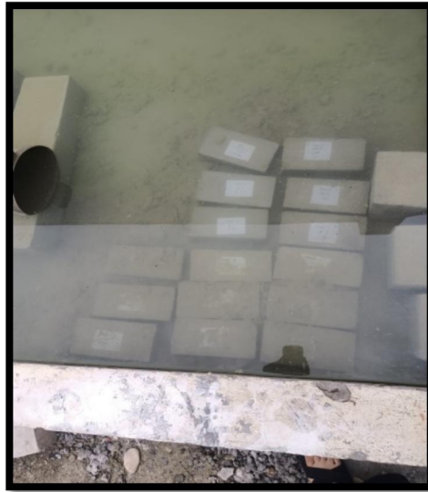
Gambar 4.17 Proses curing paving block
